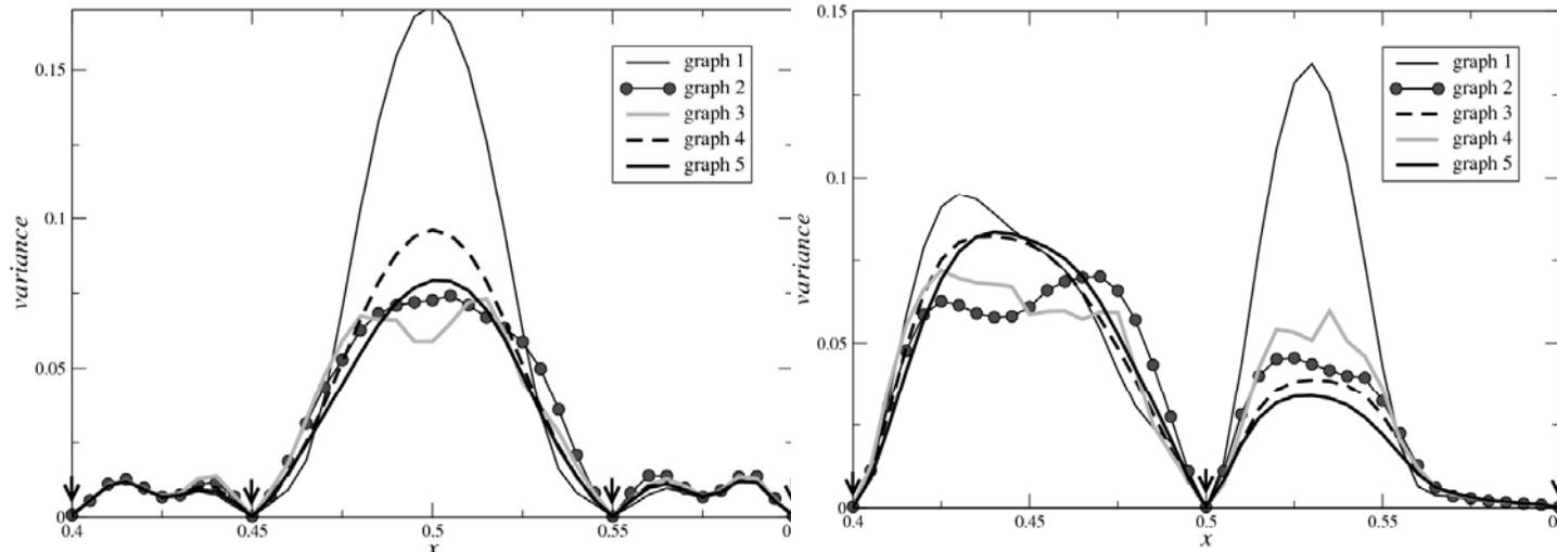
In Figures: graph 1 - inverse Hessian on exact solution, graph 2 – estimate by the fully nonlinear ensemble method ( $L=1600$ ), graph 3 (pale line) – estimate by the fully nonlinear ensemble method ( $L=50$ ) with compensation, graph 4 (dashed line) – 'effective' inverse Hessian method using sample of optimal solutions ( $L=50$ ), graph 5 (bold line) – 'effective' inverse Hessian method using sample of randomly generated functions ( $L=50$ ).
