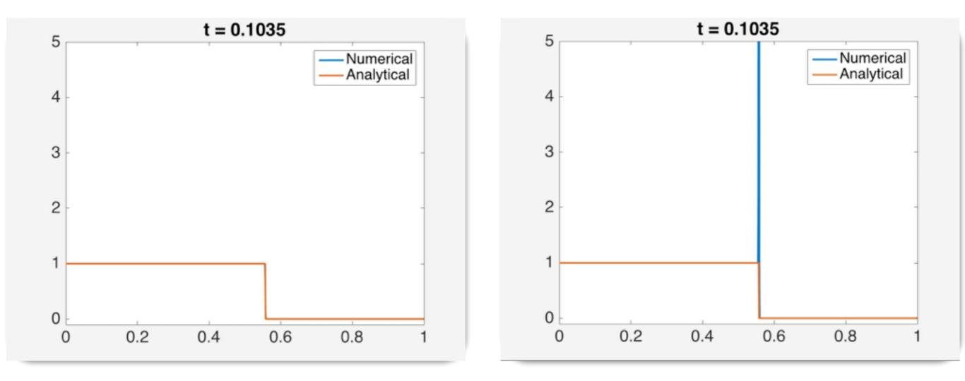
The same shock detector in a less simple case does not work:
